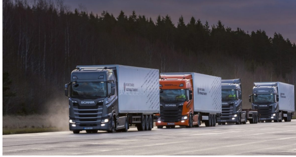
Figure 1.7. Scania platooning [image courtesy of Scania]
