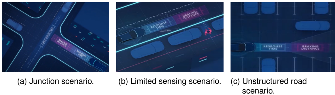
Figure 1.8: Critical navigation scenarios treated by RSS model for safety guarantees.
