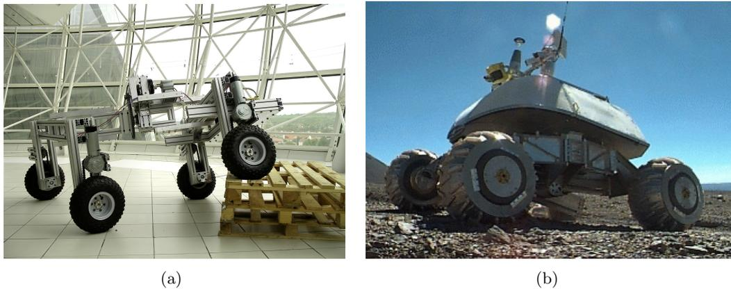
FIGURE 2.7: Wheeled mobile robots: a) OpenWheel: All terrain four wheeled robot [48]; b) Nomad: Four-wheeled robot [180]
