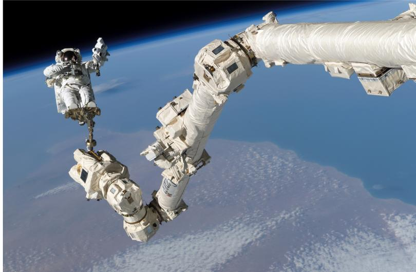
FIGURE 2.1: Station Remote Manipulator System [9]
