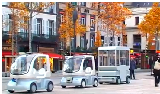
Figure VI.4: Example of autonomous navigation in formation of a group of UGVs in an urban environment (Clermont-Ferrand, France). MobiVIP project (Predit 3).
