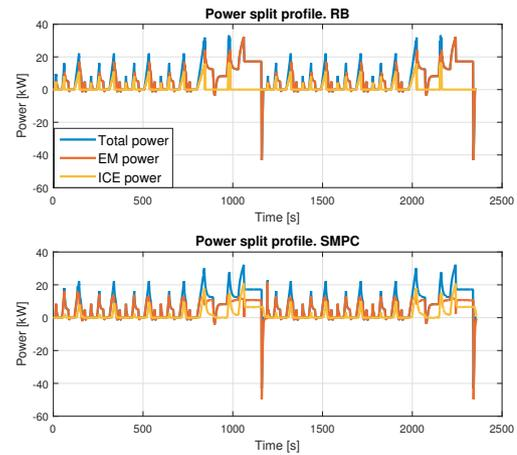
Fig. 7. Powersplit Profile for NEDC SDC
