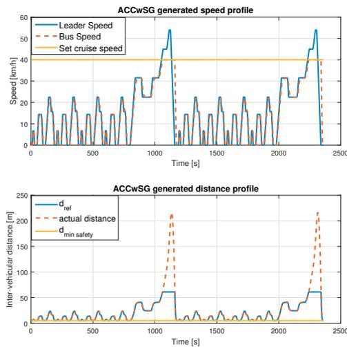
Fig. 6. Speed and Distance Profiles for NEDC SDC
