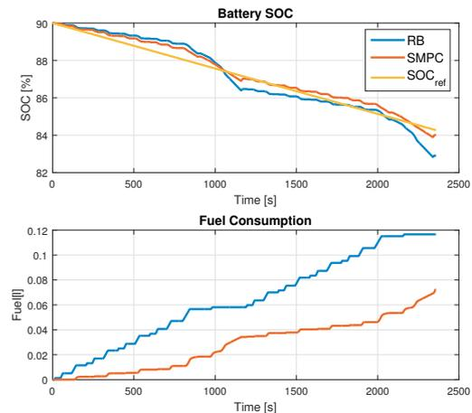
Fig. 8. SOC and fuel consumption comparison for NEDC SDC
