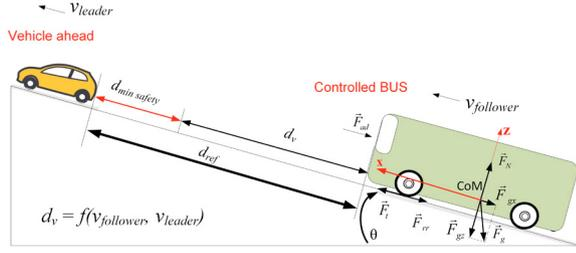
Fig. 2. Forces acting on the bus and ACCwSG scheme
