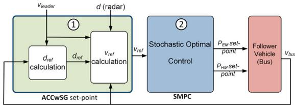
Fig. 3. Proposed global control architecture
