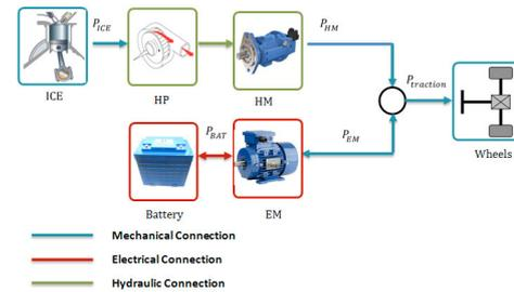
Fig. 1. Block diagram of the powertrain power flows. (ICE: internal combustion engine, HP: hydraulic pump, HM: Hydraulic motor, EM: electric motor)
