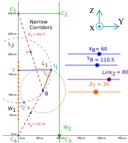
Fig. 3 Collision avoidance with wall  $C_1C_4$
