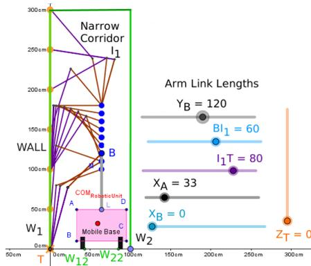
Fig. 5 Continuous wall Vertical Trajectory
