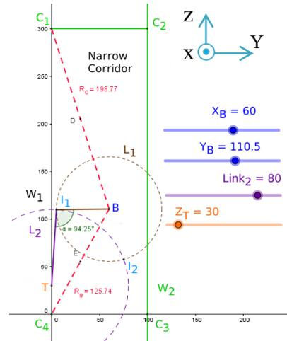
Fig. 4 Collision avoidance with wall  $C_2C_3$
