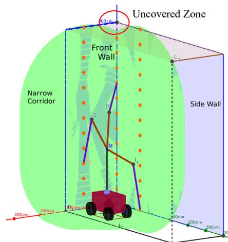
Fig. 8 Intersection of the workspace with side and front wall
