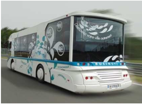
Figure 1: BUSINOVA a Hydraulic-Electric Hybrid bus.
