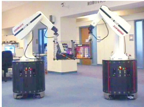
Stanford robotic platform [Khatib, 1999]: Two holonomic mobile platforms equipped with PUMA robot arms
