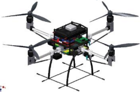
Variable pitch for 4+ rotor UAS
