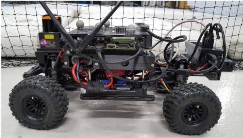
Small-Vehicles-for-Autonomy (SVEA) equipped with NVIDIA Jetson TX2 embedded computer and Qualisys motion capture system
